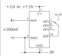
Measuring a single ended input voltage referenced to supply, i.e. the input voltage and the meter's power supply share the same OV rail. Ensure solder link LCOM is open.
