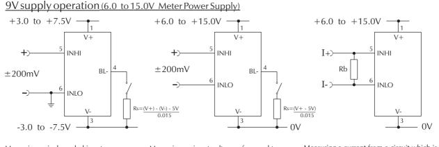
Measuring a single ended input voltage referenced to supply, i.e. the input voltage and the meter's power supply share the same OV rail. Ensure solder link LCOM is open.
