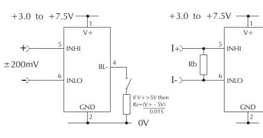
Measuring an input voltage referenced to a floating supply, i.e. the input voltage and the meter's power supply are isolated from each other. Ensure solder link LCOM is closed.
